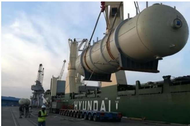
Discharged In Iraq Pressure Vessels, Convection Modules
